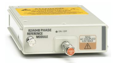
The 82A04B Phase Reference Module extends the capability of the DSA8300 Digital Serial Analyzer sampling oscilloscope 1 by providing extremely low litter/drift sample position information to the mainframe. This sample position information is based on the phase of a clock the user provides to the 82A04B input.
